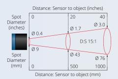
The sensor can measure at longer distances than shown, with a larger measured spot size.
